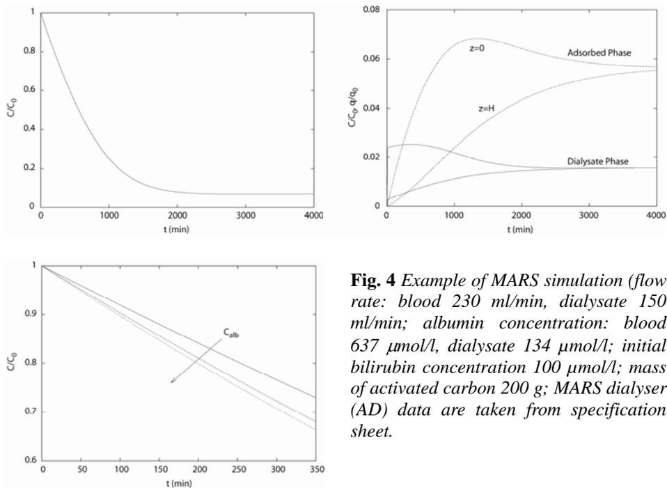
**Fig. 4** Example of MARS simulation (flow rate: blood 230 ml/min, dialysate 150 ml/min; albumin concentration: blood 637  $\mu\text{mol/l}$ , dialysate 134  $\mu\text{mol/l}$ ; initial bilirubin concentration 100  $\mu\text{mol/l}$ ; mass of activated carbon 200 g; MARS dialyser (AD) data are taken from specification sheet).
